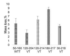
Figure 1. The ML after different thermal treatments of veneer samples.
