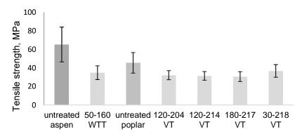
Figure 2. The tensile strength of veneer samples.
